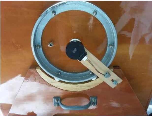
The other photo is a close-up of the encoder installation on the altitude axis. Plus I had to raise the OTA by making wood crescents to go in the original trunnion cutouts in the rocker box. The scope wasn't originally designed with having an encoder on the azimuth axis in mind. I needed to raise it by about 1.5 inches to make room for the corner of the mirror box to clear the azimuth encoder.
