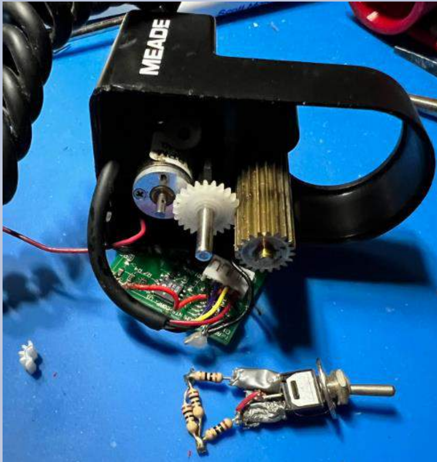
The electronic focuser with the broken spur gear (lower left) and the user added toggle switch (lower right). You can see where the motor shaft is missing the gear.
